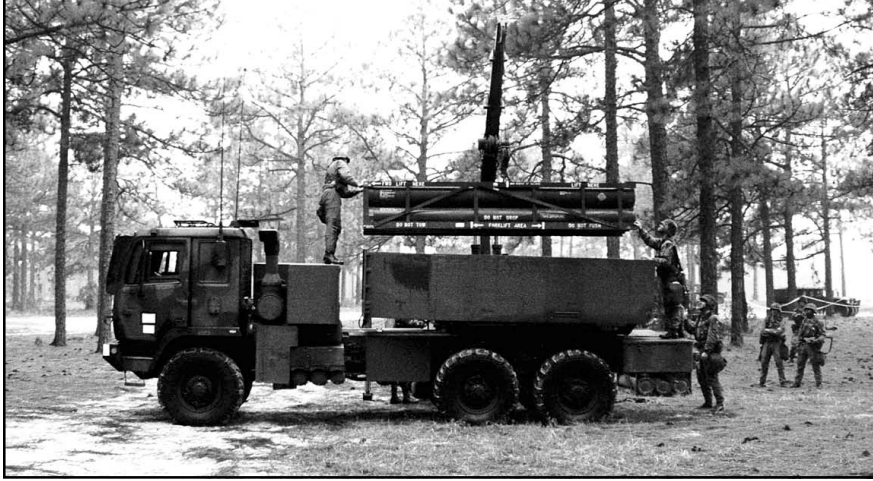
Soldiers of 3-27 FA (MLRS), part of the 18th FA Brigade, work with a high-mobility artillery rocket system (HIMARS) prototype at Fort Bragg, NC. (Photo courtesy of Lockheed Martin)
